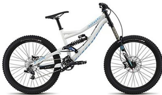
Mountain Bikes are generally used for off-road riding and rougher terrain. Key features include wider tires with a thicker tread to provide increased traction, and suspension systems designed to absorb shock. These bikes tend to be heavier because of their robust construction and suspension components.
