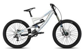
Mountain Bikes are generally used for off-road riding and rougher terrain. Key features include wider tires with a thicker tread to provide increased traction, and suspension systems designed to absorb shock. These bikes tend to be heavier because of their robust construction and suspension components.
